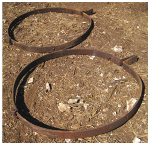
Fig. 54: The two hoops used to secure columns in 1880, seen in the Bassai archaeological site in 2012.
