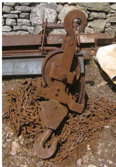
Fig. 60: The lifting mechanism used in the conservation work of 1965 and 1966, seen in the Bassai archaeological site in 2012.
